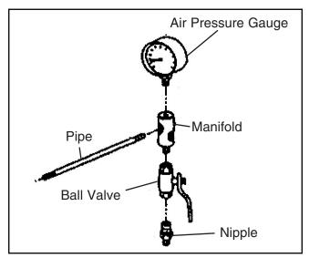
Figure 5. Gauge/air supply control installation.
